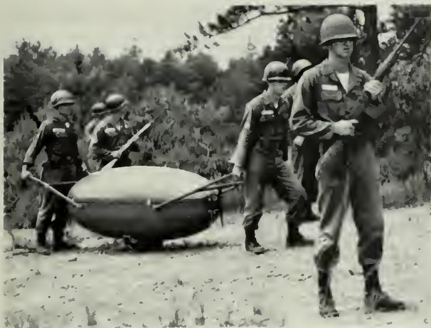
LOAD CARRYING device being tested by Army was designed for use as supply carrier for small units in normally inaccessible areas. Fiber glass cart has wide wheel for land use, can be opened into two-man boat as needed.
